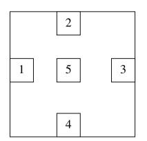
Figure 5. Fiducial distribution on a KFA-1000 photo
